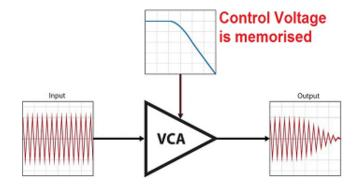
As the control voltage is really just a stream of numbers it is easy to record "**write**" your fader or dial movements, and even "**update**" the movements, and finally save all your movements as a file. Any time you wish you can ask the Automation system to "**read**" its' memory and send back those control voltages exactly as the controller (fader or dial) was moved, and it can repeat this whenever you want.
