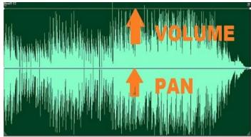
Software packages display lines over top of the Audio tracks. A line might represent the memorised positions of the Fader (volume), one might be the memorised positions of the Pan (L-R), and another might be the Mute for that channel. Initially they will be straight lines, until you memorise some changes.
